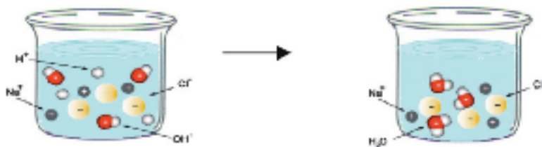
Figure 1 Particles before and after a strong acid – strong alkali neutralisation reaction. (Adapted from British Columbia Institute of Technology website: http://www.bcit.ca )
