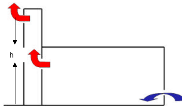
Figure 1(d) Stack ventilation: one front façade opening, one transfer vent on the back wall into a stack
