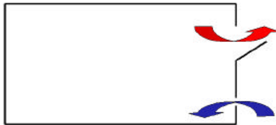
Figure 1(b) Single side ventilation: a single low level vent and one openable window
