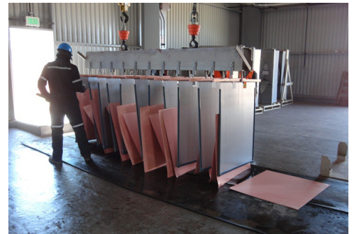
Copper is stripped from the steel cathode plates when it is thick enough. This cathode copper is 99.99% pure.
