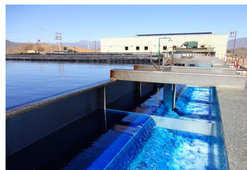
After solvent extraction using organic solvents, the copper ions are stripped from the solution with a strong acid and leave a blue solution with a high copper content. This is called the 'rich electrolyte'. (Courtesy of Red Tiger Mining Inc.)
