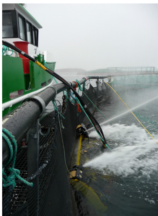
A support ship operates a remote control net washing machine. Cleaning is an expensive operation. (Courtesy of Aurora.)
