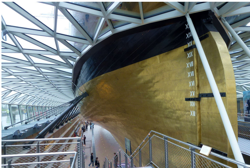
Hull of the restored tea clipper, Cutty Sark, clad with Muntz metal, originally fitted to prevent biofouling and optimise speed. (Wikimedia CC Cmglee.)
