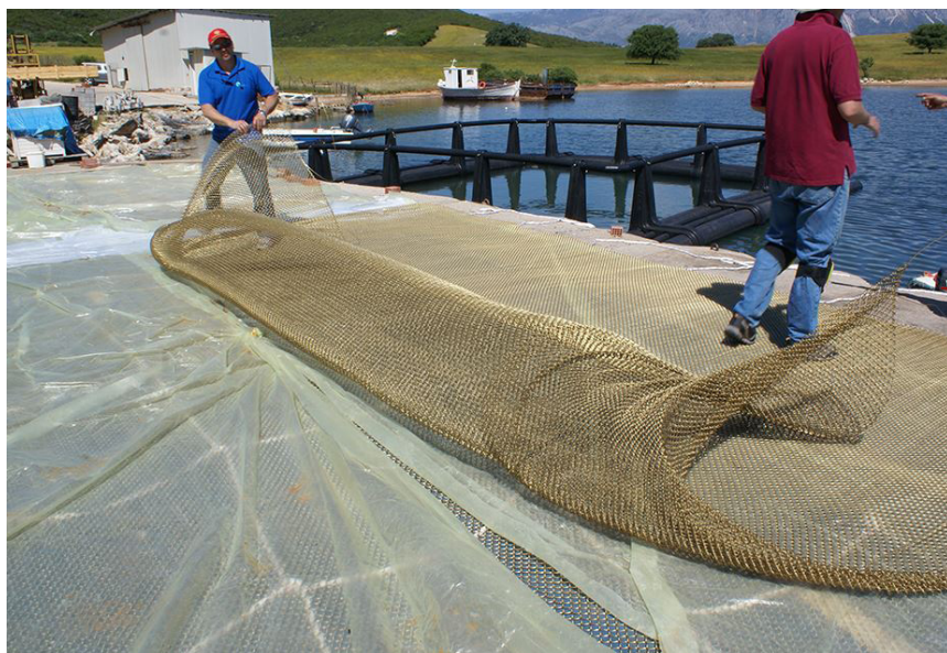
The image above shows copper alloy mesh being made into pens in Greece by the aquaculture company Nireus. This is part of a global research programme to test copper alloy mesh pens. (Courtesy of Nireus.)
