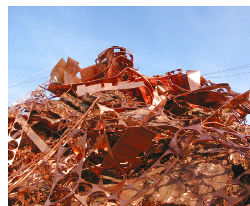
Process scrap, or 'new scrap', comes directly from manufacturers and has a very high value. (Courtesy of Aurubis.)
