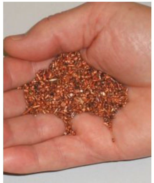
Granules of copper formed after chopping up the kilometres of copper cabling.
