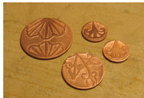
The flower patterns on these jewellery discs were painted with a lacquer that resists ferric chloride. The exposed areas have been partly dissolved by the ferric chloride, leaving a raised pattern. (Courtesy of Copperheart.)
