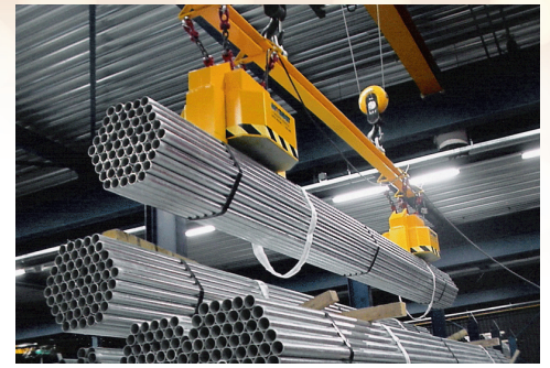
Lifting magnets can lift and drop heavy loads like this steel pipe without the need for anyone on the ground fixing ropes, making the process safer. (Courtesy of Directindustry.)
