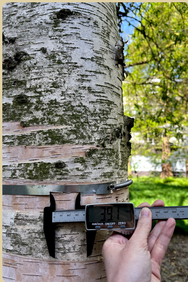
Figure 2 A dendrometer band installed for the BIFoR in a Box project; tree growth measurements are taken using a digital caliper
