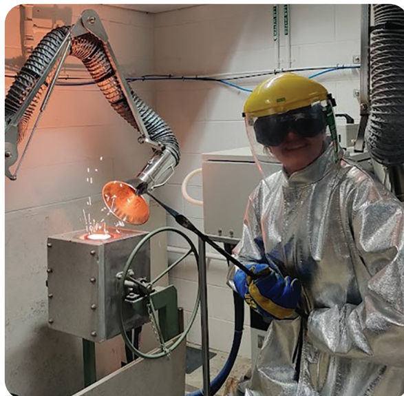
Sampling steel in the induction furnace at 1630 °C
